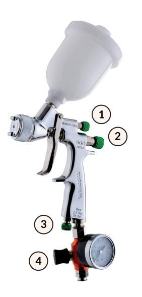
From 0 to 5 turns of opening for a micrometric and ideal setting of the fan according to your needs. MATERIAL FLOW (2) CONTROL From 0 to 5 opening turns for a micrometric and ideal setting of the product delivery based on the paint and the speed of the operator. AIR (3) ADJUSTMENT Completely open for total air flow. AIR INLET (4) PRESSURE Usage range 0.5 - 2.5 bar
